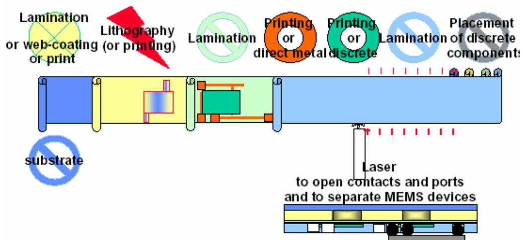
**Fig. 4. Reel-to-reel processing of low-cost MEMS**
