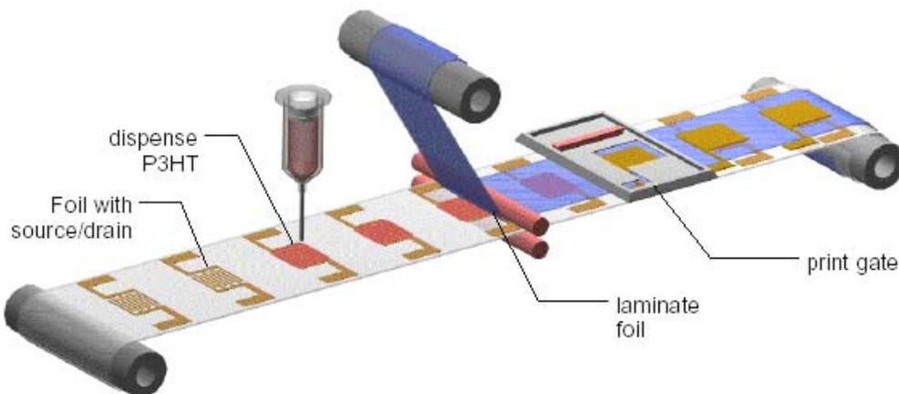
**Fig.3. Reel-to-reel processing of Polymer Transistor**
