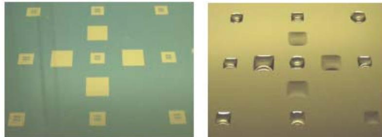
**Fig. 5. Self assembly systems - assembly pattern on silicon by hydrophilization; layout for hydrophilization (left) and plasma hydrophilized Si-chip wetted with water (right)**
