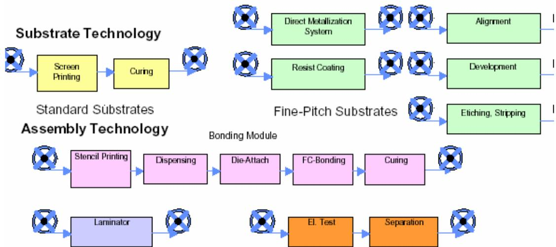
**Fig.2. Modules of the Reel to Reel Application Center at IZM Munich**
