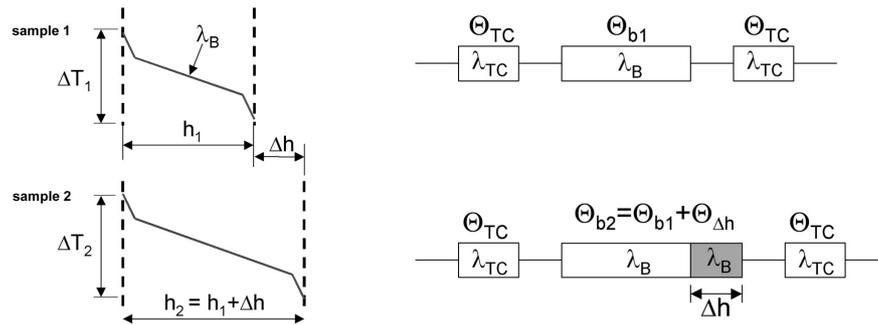
Fig. 3. Temperature profiles and equivalent thermal circuits for samples with different thicknesses;  $\lambda_{TC}$  is thermal conductivity of thermal contact;  $\lambda_B$  is thermal conductivity of tested material
