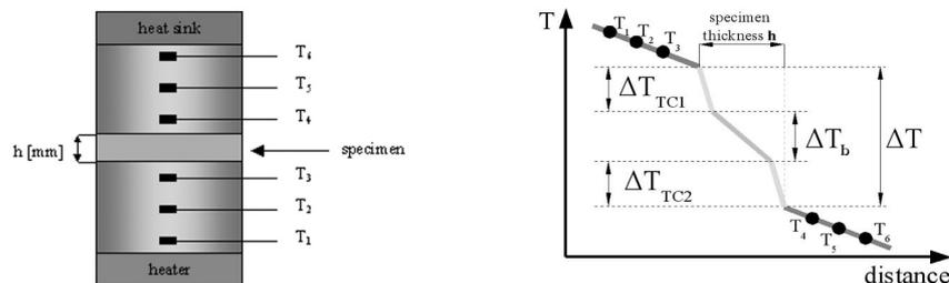
Fig. 2. An experimental setup and thermal distribution in steady state.
