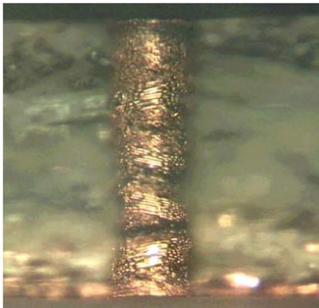
Through hole with 0.3 mm diameter
