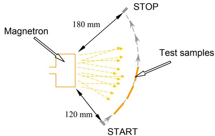
Fig. 2. The movement of test samples during the magnetron sputtering process
