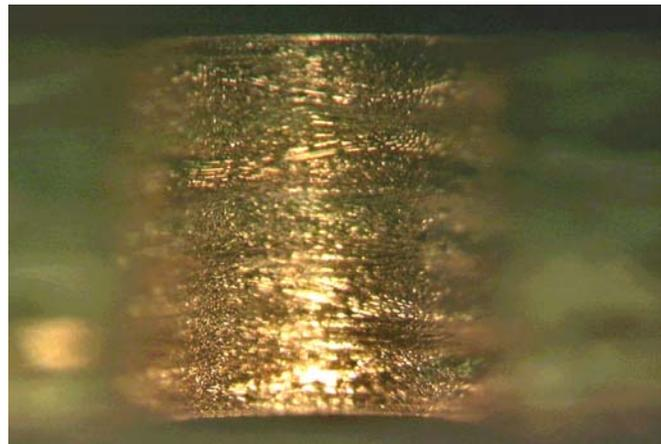
Through hole with 1.0 mm diameter
