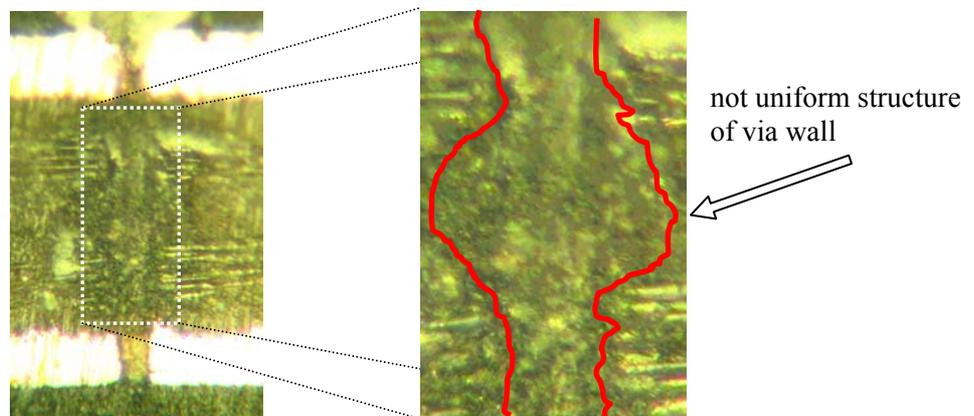
Fig. 1. The first trials of magnetron sputtering metallization of laser drilled microvias in FR-4 material (50  $\mu\text{m}$  diameter on the top of via)
