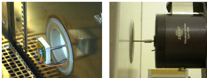
Figure 3. The vibration system inside (left) and outside (right) a climatic chamber
