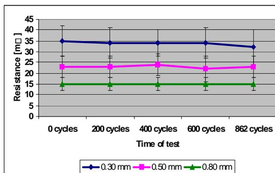
Fig.2 Tube shape fill resistance changes during thermal shock tests
