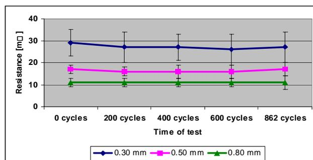
Fig.1 Full fill resistance changes during thermal shock tests
