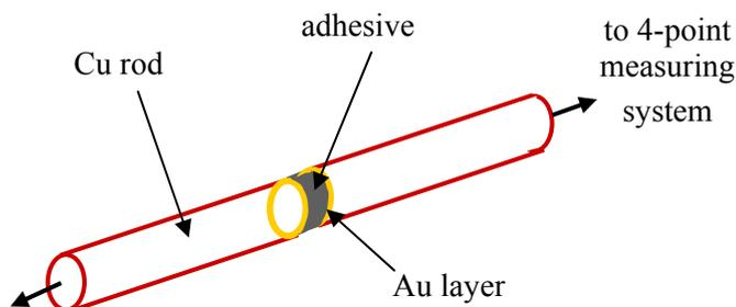
Fig. 4. Four-point probe configurations.
