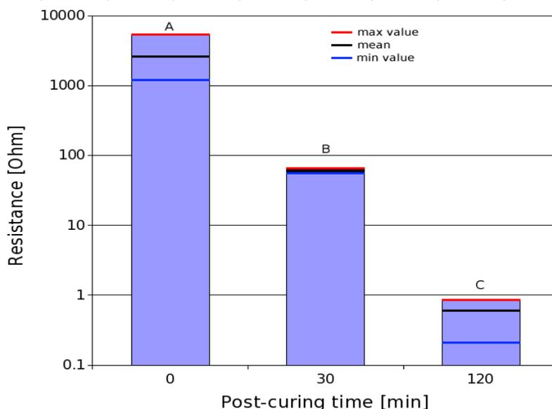
Fig. 5. The adhesive joint resistances vs. post-curing processes time
