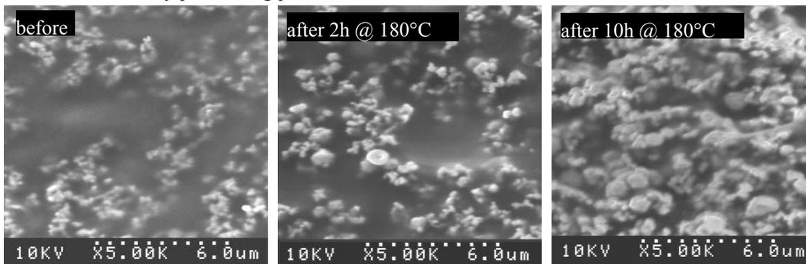
Fig. 2. SEM images of surface of epoxy resin with Ag powder filler formulation before and after 2h and 10h in 180°C post-curing process.
