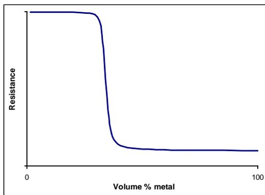
Fig. 1. Generalized percolation curve showing the abrupt drop in resistance at the percolation threshold
