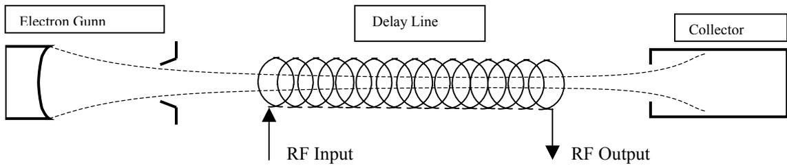
Figure 1. Simplified structure of TWT.
