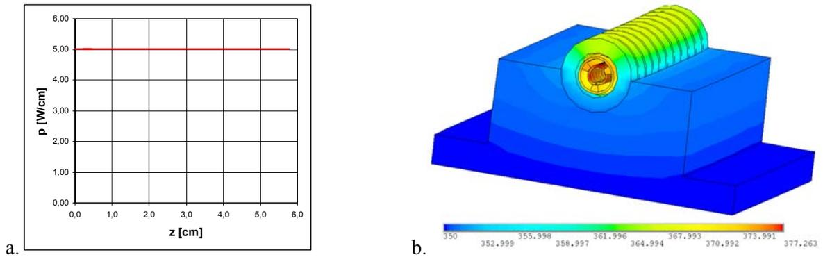
Figure 4. The results for uniform power dissipation (a) and the corresponding temperature distribution (b).
