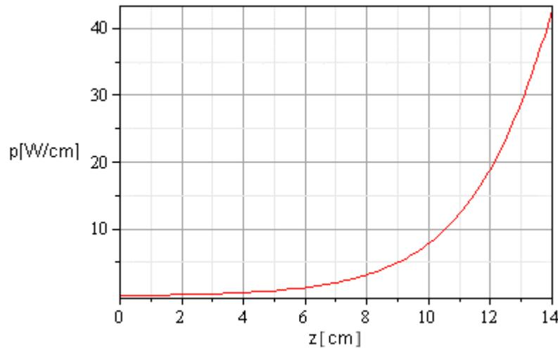
Figure 3. Linear power density dissipated in the delay line of designed TWT.
