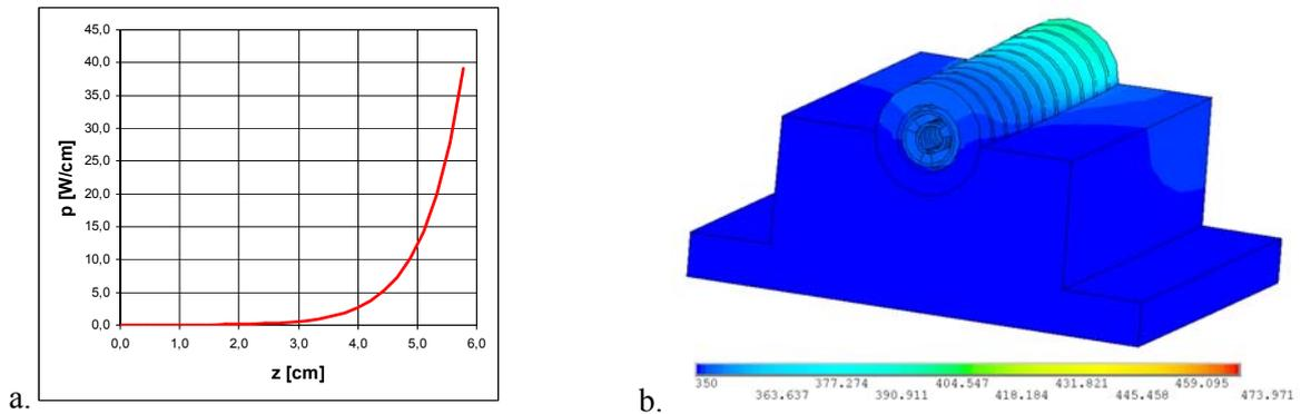
Figure 5. The results for non-uniform power dissipation (a) and corresponding temperature distribution (b).
