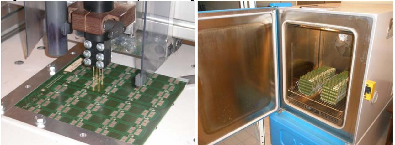
**Figure 1.** View of the test PCB and the climatic chamber
