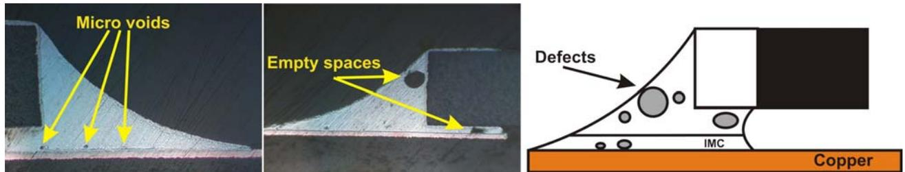
Figure 1. Examples of detected defects of solder joint structures considered during evaluations and Anova analysis
