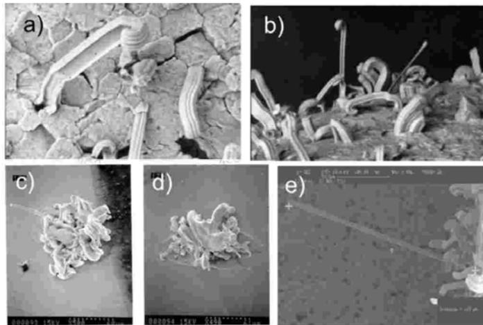
Figure 1. Various whisker shapes a) bent, b). kinked, c), d) odd-shaped, e) needle whisker [6].
