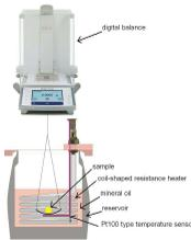
Figure 7: The measuring set up
