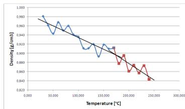
Figure 6: Change of density in the function of temperature for mesoscale
