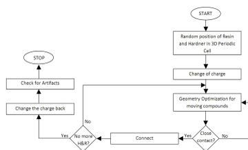
Figure 1: Algorithm of connecting resin and hardner
