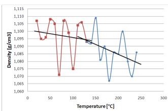
Figure 4: Change of density in the function of temperature
