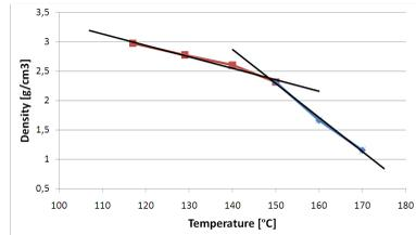
Figure 9: The change of the density in the function of temperature for SIQ resin
