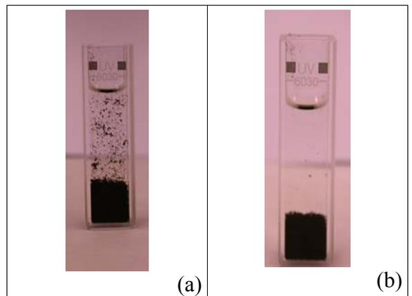
Fig. 7: Shelf test for CNTs dispersed in acetone; (a) just after preparation of suspension and (b) after thirty minutes on shelf.
