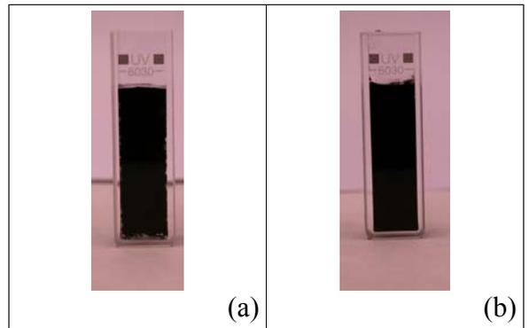
Fig. 6: Shelf test for CNTs dispersed in distilled water; (a) just after preparation of suspension and (b) after thirty minutes on shelf.
