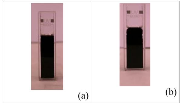
Fig. 5: Shelf test for CNTs dispersed in isopropyl alcohol; (a) just after preparation of suspension and (b) after thirty minutes on shelf.
