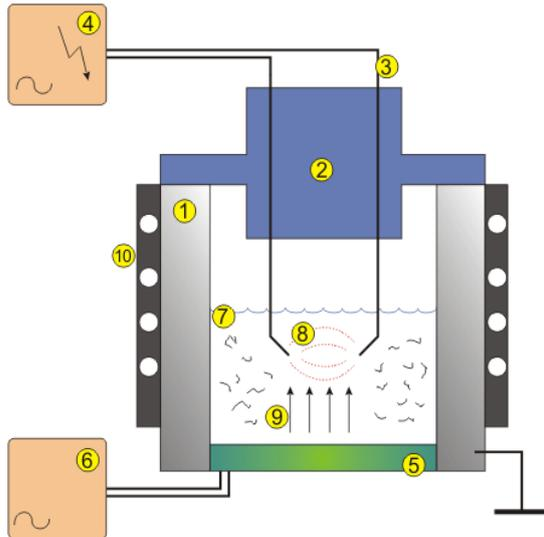
Fig. 1: Diagram of chamber for efficient CNTs dispersion, (1) the chamber made of stainless steel, (2) the cover made of polytetrafluoroethylen, (3) electrodes, (4) the power supply, (5) the ultrasonic/megasonic transducer, (6) the control/driver unit for transducer, (7) the fluid with carbon nanotube, (8) the electric field, (9) the acoustic wave from transducer, (10) the heater/heat - sink.
